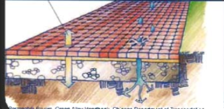
Permeable Pavers, Green Alley Handbook, Chicago Department of Transportation
