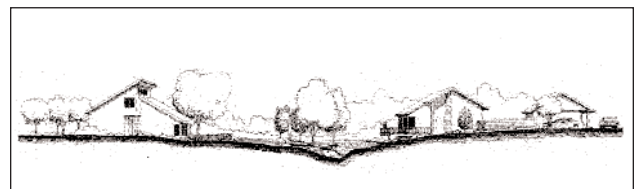
Naturalized back yard drainage swales provide public open space, habitat and stormwater retention. (Village Homes, Davis, CA)
