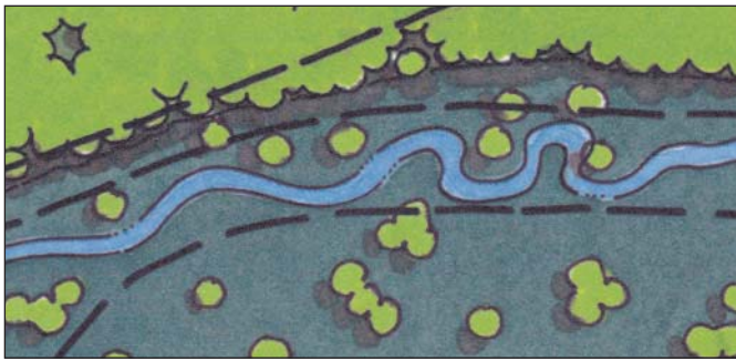
Re-Meandered Stream for habitat and restoration of natural stream-floodplain relationship.
